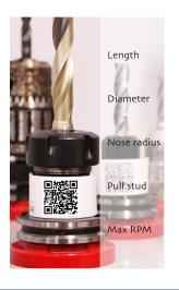
A single scan transmits all tool data to the correct fields in the CNC control
