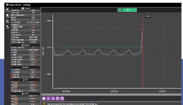
TMAC Data Viewer – shows successfully drilled holes with the last one generating an extreme alarm indicating tool breakage.
