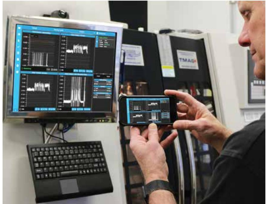
Blum-Novotest's Tool Monitoring Adaptive Control TMAC 3.0 monitors tool wear and breakage and sends a notification or stops the machine if necessary.
