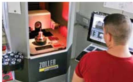
Zoller's genius 3 is a universal measuring machine capable of logging measurement details and allows the operator to transfer data directly to machines instantaneously.
